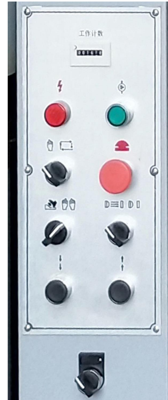
Work control panel
